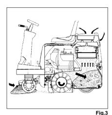
Principle of Sweepmaster P980 R The side brush is used to collect dirt at borders and to enlarge the working width as well as to increase the area performance on large surfaces.
