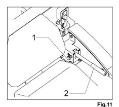
Release lever, swing dirt hopper
