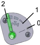
Make sure that the adjusting lever has been opened sufficiently. Water supply only starts from mark (1) onwards!
