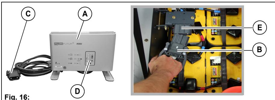
The batteries are charged with the charger **Fig. 16-A**. The batteries can already be charged when one segment in the charging status indicator **Fig. 14-51** has gone out.
