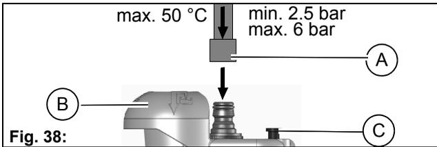
1. Fit the water connection **Fig. 38-A**. Do not yet open the water supply!
