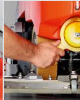
Overview at a glance: Wear indicator for brushes and pads. A comfortable discharge system enables fast and easy changing of the brushes – without the need for tools.
